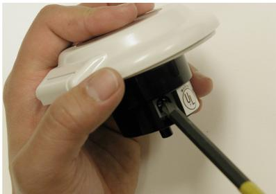
4. Back off terminal screws on the rear housing of the inlet. Insert wires into color coded openings on the back of the inlet. Tighten terminal screws to 14-20 in.-lbs. torque. **Make certain there is no wire insulation under any terminal and the gasket is in place. Note: Two gaskets provided, use the gasket that best fits your installation**
