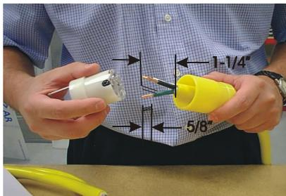
4. Strip outer jacket of cord 1-1/4 in. and 5/8 in. of insulation off each of the three wires. Cut away filler. Make sure the wire is clean and with bright copper color. Do not solder the ends of the wire.
