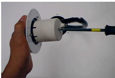
5. Slide the rear safety enclosure onto the back of the inlet. Note: The rear safety enclosure has slots on the sides that must align with the tab on the back of the inlet. The rear safety enclosure can be attached in 8 different positions. Attach the rear safety enclosure to the inlet with the center set screw. Tighten the strain relief clamp screw until it is snug around the wiring.
