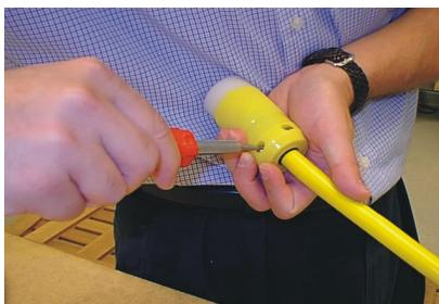
8. Tighten cord clamp by tighten two assembly screws to 16-20 in.-lbs torque.
