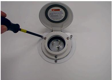
6. Position the gasket and inlet over the adapter mounting bracket. There are two brackets provided. Choose the appropriate mounting bracket based on the size of the hole. Align the mounting holes and tighten the screws to 5-7 in.-lbs. torque with provided 8-32 screws. Fasten the mounting bracket to existing mounting holes.
