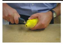
**1.** Cut boot at first line for cable greater than 10/3. Invert tapered end of the boot and apply soap solution.
