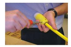
**8.** Tighten cord clamp by tighten two assembly screws to 16-20 in.-lbs torque.
