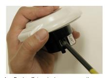
4. Back off terminal screws on the rear housing of the inlet. Insert wires into color coded openings on the back of the inlet. Tighten terminal screws to 14-20 in.-lbs. torque. Make certain there is no wire insulation under any terminal and the gasket is in place. Note: Two gaskets provided, use the gasket that best fits your installation
